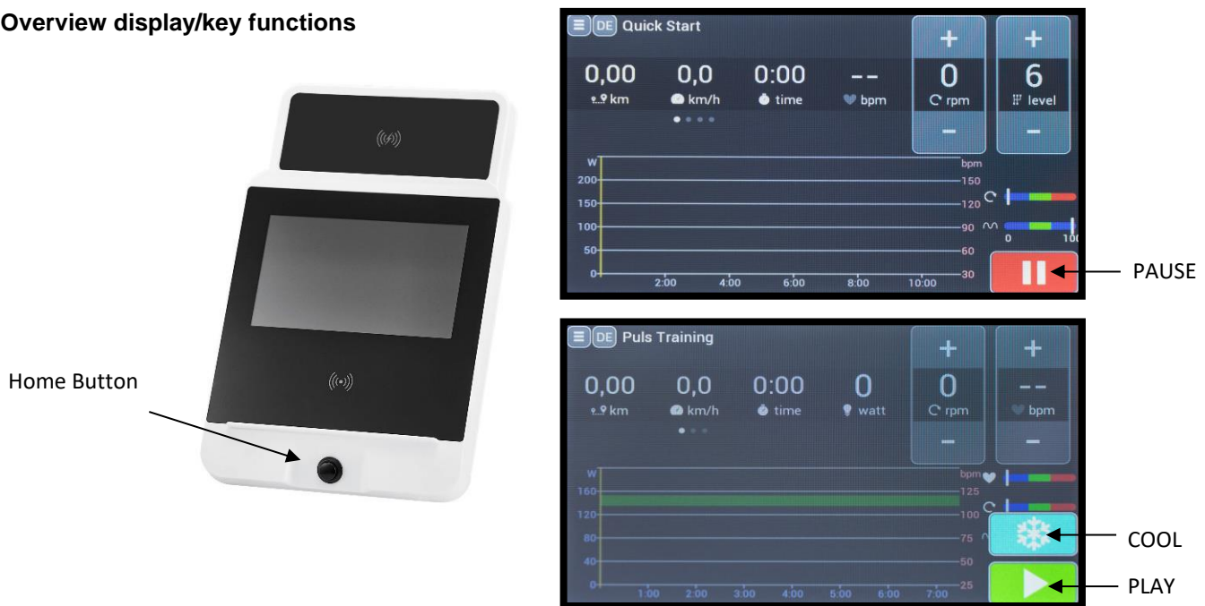
Fig. 9: Monitor view, explaining the button functions, actual view may vary in colour, button assignment is the same.
