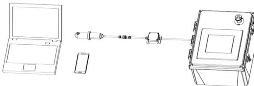
Figure 5. Bluetooth connection to HM-500 Series sensor
