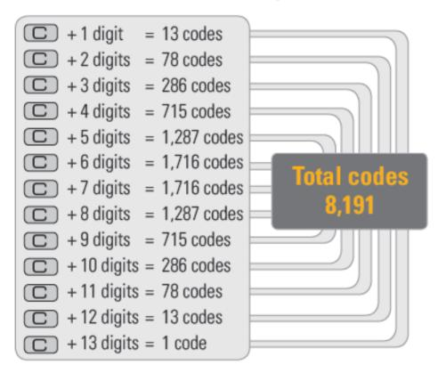
Generally codes are set in the range of 4 to 7 digits, and the total number of codes in this range is 5434. The lock is factory set with a randomly selected 6 digit code starting with the 'C' button. The code is not recorded by the factory. The code can be changed as often as required to any other 6 digit code. Every new code must start with the 'C' button. Using the spare tumblers, the code length can be changed to 5 or 7 digits. Shorter codes are not recommended.
