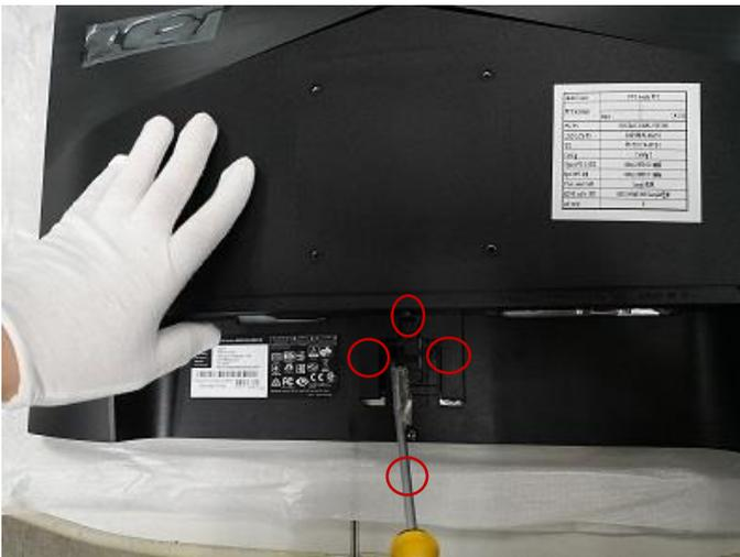
Step.3 Separate hooks between MID\_FRAME and R/C
