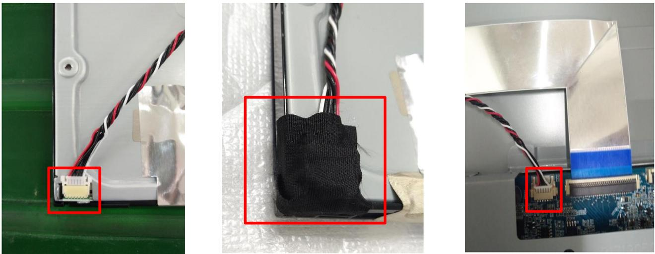
Step6. Insert 30 pin LVDS FFC to main board. Use AL tape to fix. (Tape in blue circle).
