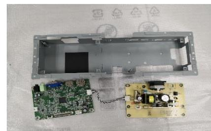
Step.8 Remove connector cable and separate main board and power board, separate Mylar and shielding
