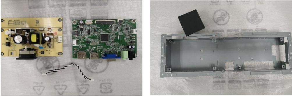
Step.9 Unscrew eleven screws and separate MID FRAME and LCM
