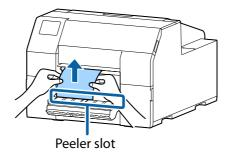
**3** Hold down the Feed button until the paper is completely ejected.
