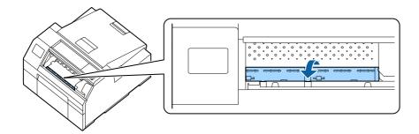
■ Use a cloth or cotton swab to remove adhesive adhered to the platen.
