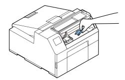
If the print head is not on the far right, hold it down and move it to the far right. If there is jammed paper on the position that the print head was stopped, remove it.
