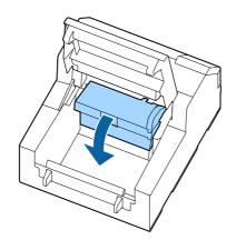
Attach adhesive side of a label to the roller, and peel it off slowly. Repeat this action until paper dust or adhesive is completely removed from side to side of the roller. If some labels have stuck on the roller, carefully remove them as they can cause a paper jam.
