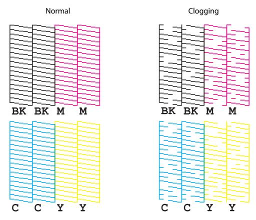
If nozzles are clogged, run a print head cleaning. Run [Power Cleaning] only when nozzle clog is not cleared by running [Print Head Cleaning].
