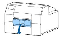
Cut the paper near the paper ejection slot.
