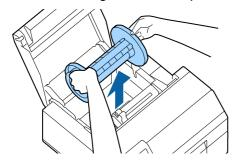
**1** Raise the paper guide unit, and then remove any jammed paper from the inside.
