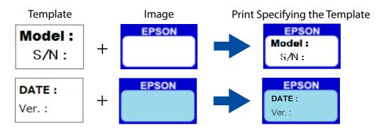
First store the image and the template data in the printer, and then make the link setting.
