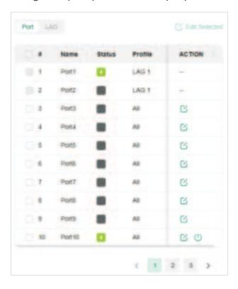
Select the profile from the drop-down list to assign the port profile to the desired ports
