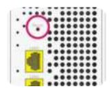
3. Withdraw the paperclip. LED on the front panel displays blinking red to indicate factory reset in progress
