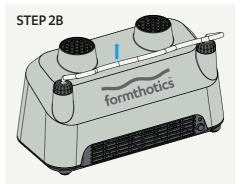
Adjust the shoe rest bar to an appropriate height.
