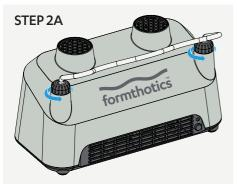
Loosen the shoe rest bar twist locks with a half turn anti-clockwise.
