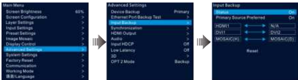
Figure 5-33 Input source backup
