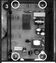
Unplug all 6 wires from connection terminals and remove 4 screws.
