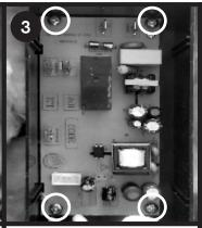
Unplug all 6 wires from connection terminals and remove 4 screws.
