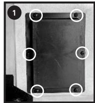
Remove 6 screws and PCB shield. The shield is located on the bottom of the smoker.
