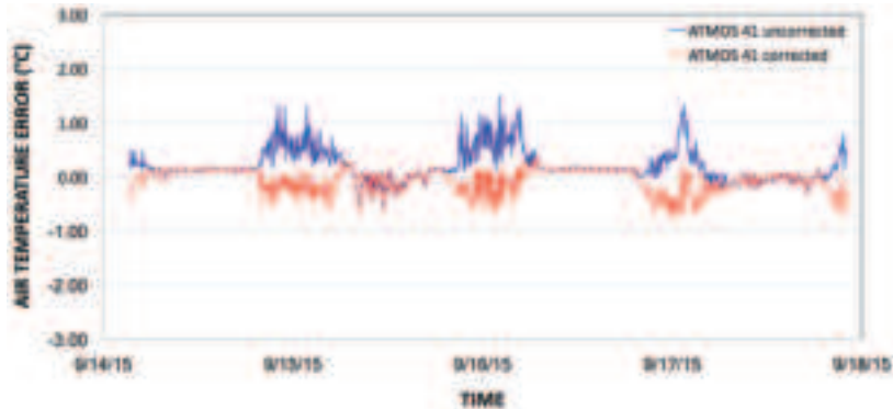
Figure 18 Corrected air temperature comparison with the aspirated radiation shield using 1-min measurement intervals
