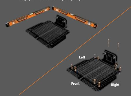
osition & Connect the Charging Station Position the charging station so Vision can enter it from a counterclockwise path.
