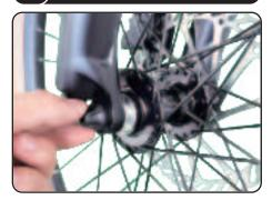
Hold the nut on one side andtighten the nut on the other side of the wheel onto the fork.
