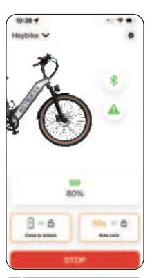
The Bluetooth icon on the main page will stay firm green which means the APP is connected successfully with the bike. (Note: the blinking blue Bluetooth icon means the APP doesn't connect with the bike)
