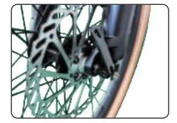
Ensure the front wheel and quick-release lever are properly secured before moving on to the
