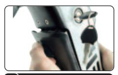
Hold the bike frame with your right hand, locate the locking device on the battery with your left hand then turn anticlockwise.
