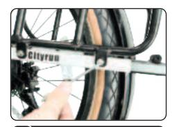
Hold the rack onto the bike frame and tighten the rack with the screw
