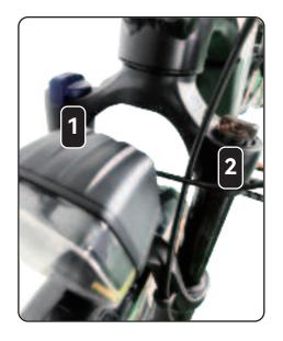
**The preload adjustment knob (2)**, located on the top of the left side of the suspensionfork. To soften the ride, subtract resistance by turning the preload adjustment knob counterclockwise, in the direction of the small "-" on the knob. To make the suspension stiffer when going over bumps, add resistance by turning the preload adjustment knob clockwise, in the direction of the small "+" on the knob.
