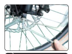
Tighten the screws on the each side of the front wheel.
