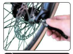
Line up the fork with the axle at the center of the wheel. Make sure there's a spacer between the fork and wheel on each side. The disc brake is on the left.
