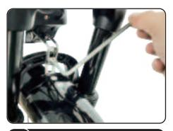
Hold the front fender and the headlight onto the bike frame and tighten them with the screw.
