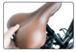
Move the seat up and down by sliding the seatpost in or out of the seat tube. DO NOT raise the seatpost beyond the minimum insertion marking etched into the seatpost
