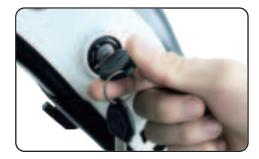
The battery can be charged off the bike. To remove the battery, turn the key to the UNLOCK position (see the previous remove battery section for details), Then carefully pull the battery up until the battery detaches from the receptacle.
