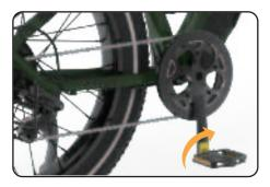
Thread the right pedal onto the right crank gently by hand, turning clockwise. Then tighten pedal by allen wrench.
