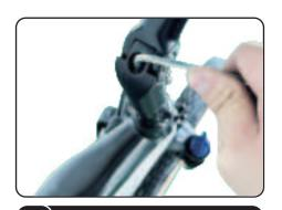
Adjust the handlebar height to your need and tighten the Allen screws on the stem.
