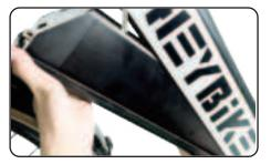
Prop up the battery with your left hand and then remove the battery with both hands. Note: the battery weighs 9.45 lbs and should be handled with care.
