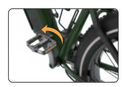
Thread the left pedal onto the left crank gently by hand, turning counter-clockwise. Then tighten pedal by allen wrench.
