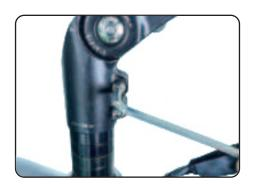
Use the wrench to tighten the screw and fix the handlebar stem in place. Check it again to make sure the handlebar stem is in line with the top tube, then use the wrench to tighten the screw and fix the handlebar stem in place.
