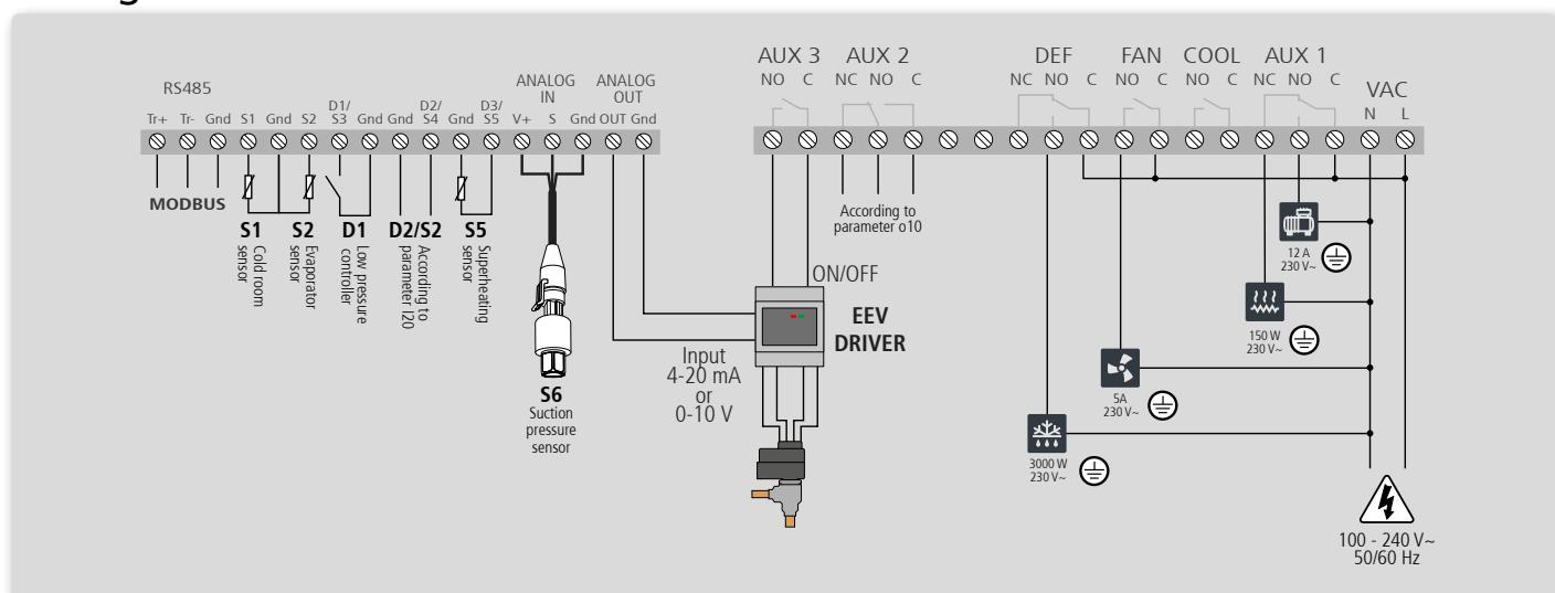
**!** The function of the D2/S4 input depends on the configuration of parameter I20.
