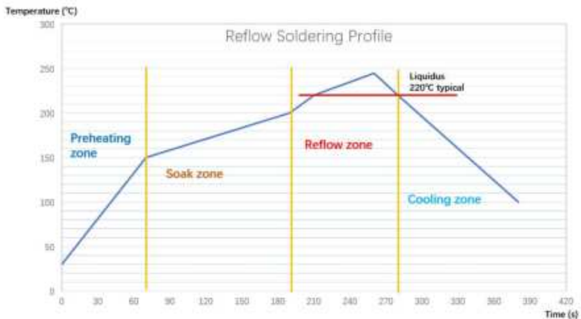
Figure 8: Temperature-Time Profile for Reflow Soldering
