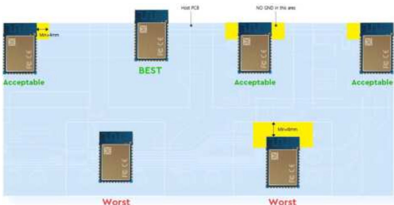
Figure 7: Recommended Module Mounting Examples
