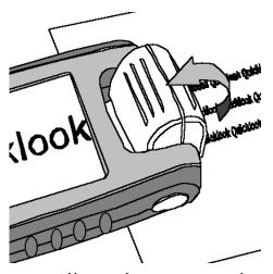
to position the **camera** directly over the area of interest. In this respect Quicklook Zoom differs from a magnifying glass in that the image you see does not correspond to the area directly beneath.
