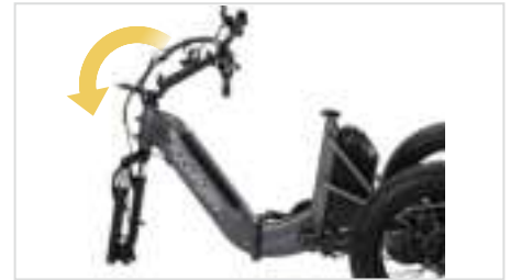
3. Rotate the handlebar upwards until it fits the frame perfectly
