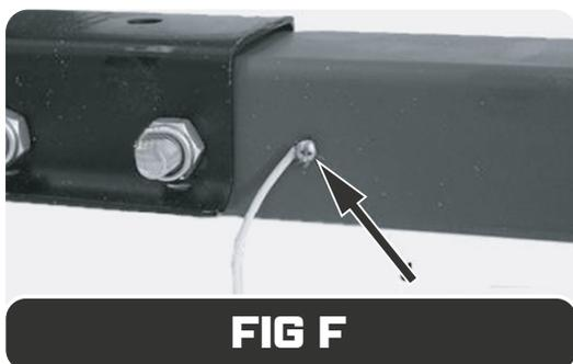
7. Run the yellow/brown wires along the inside of the front cross member to the side running light on the front left (driver) side rail.
