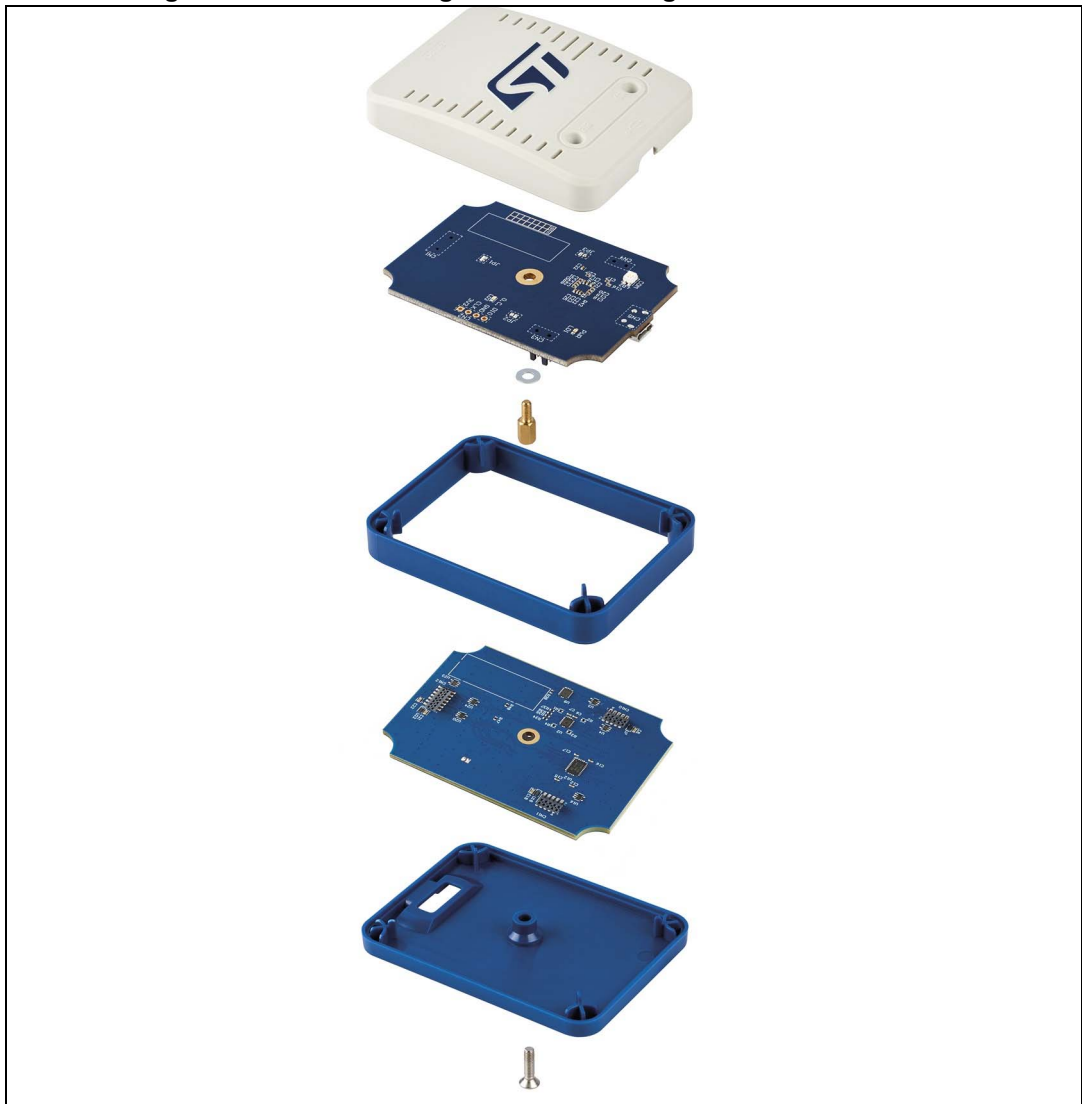
Figure 16. Closed casing for STM32 debug with B-STLINK-VOLT
