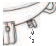
Drain valve (open)
