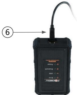
Figure 2-7 Bottom View of VCI
