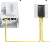
\*Must use the supplied PoE plug for power source. Other PoE plugs or PoE switches might not comply with our device.
