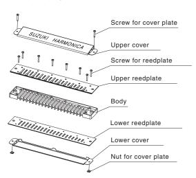
It is important to re-assemble the Harmonica so that there are no gaps in each part. Carefully check the body and reed plate, reed plate and cover, etc., and re-assemble so that there are no gaps due to particles or misalignment. The reed plate and cover are slightly curved so that they can be assembled without gaps.
