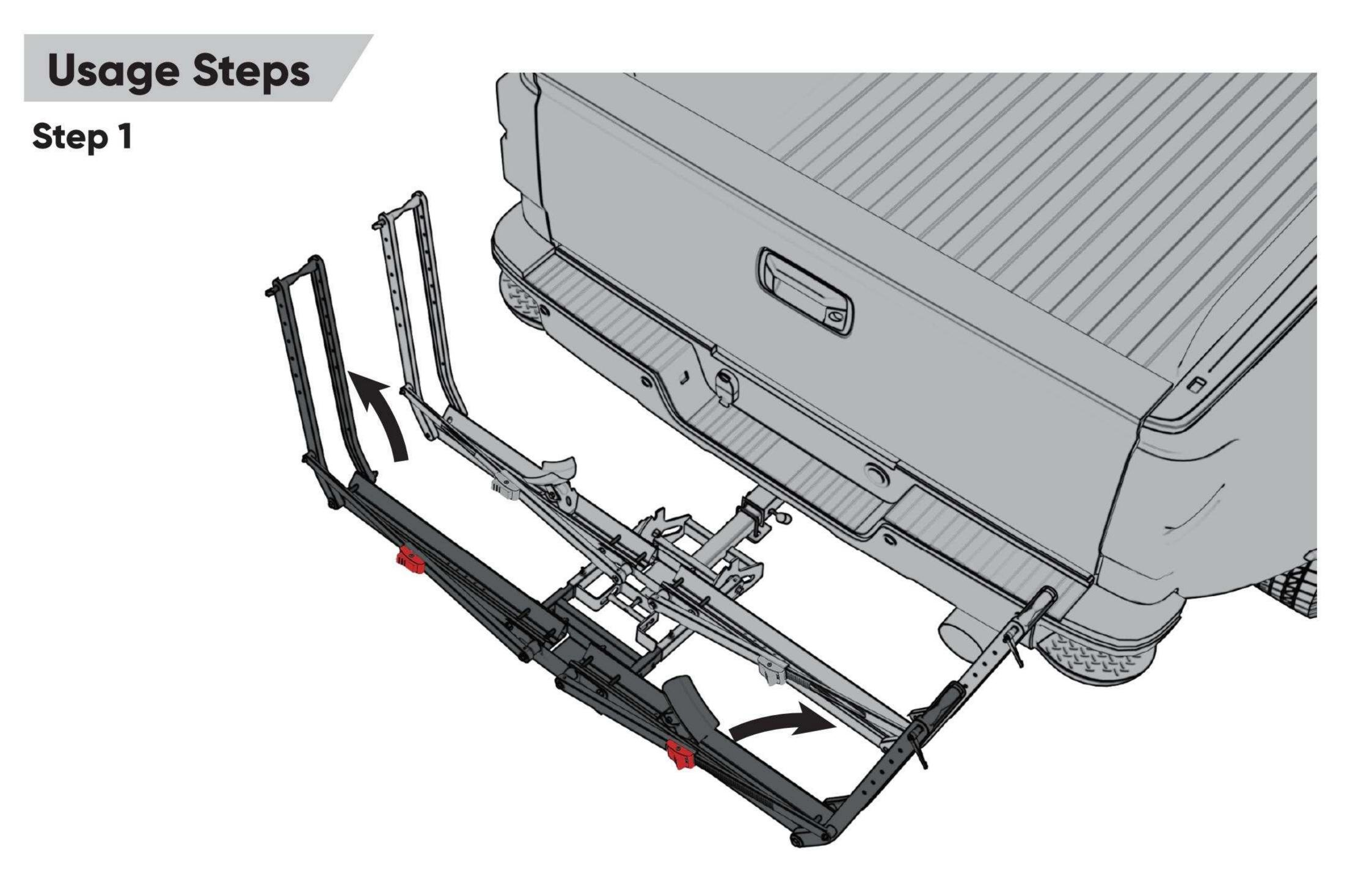
Press the Adjustment Button to unfold the Bent Arm in the direction shown in the picture.
