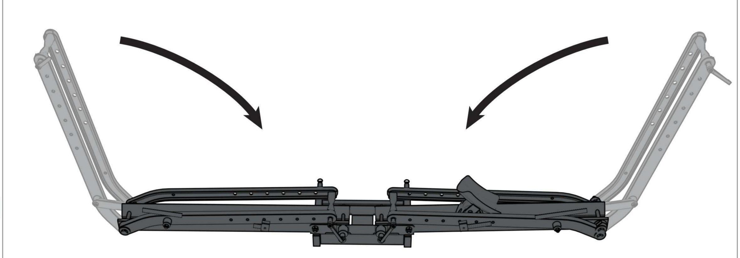
No need to press Adjustment Button when folding the bent arm assembly.
