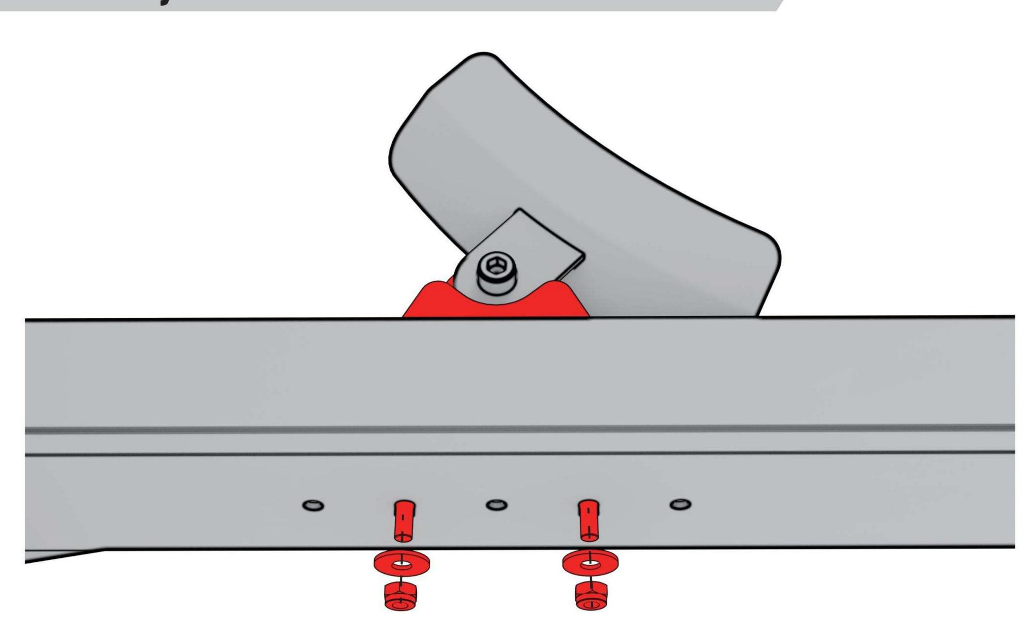
The position of the Front Wheel Holder can be adjusted according to your needs. There are three optional positions.
