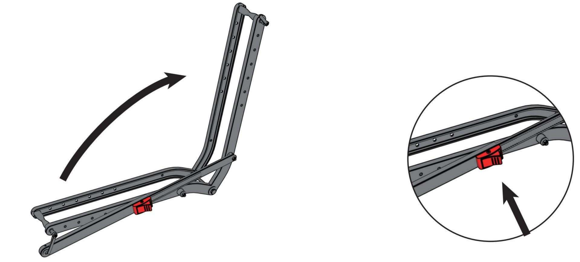
Press the Adjustment Button to unfold the Bent Arm in the direction shown in the picture.
