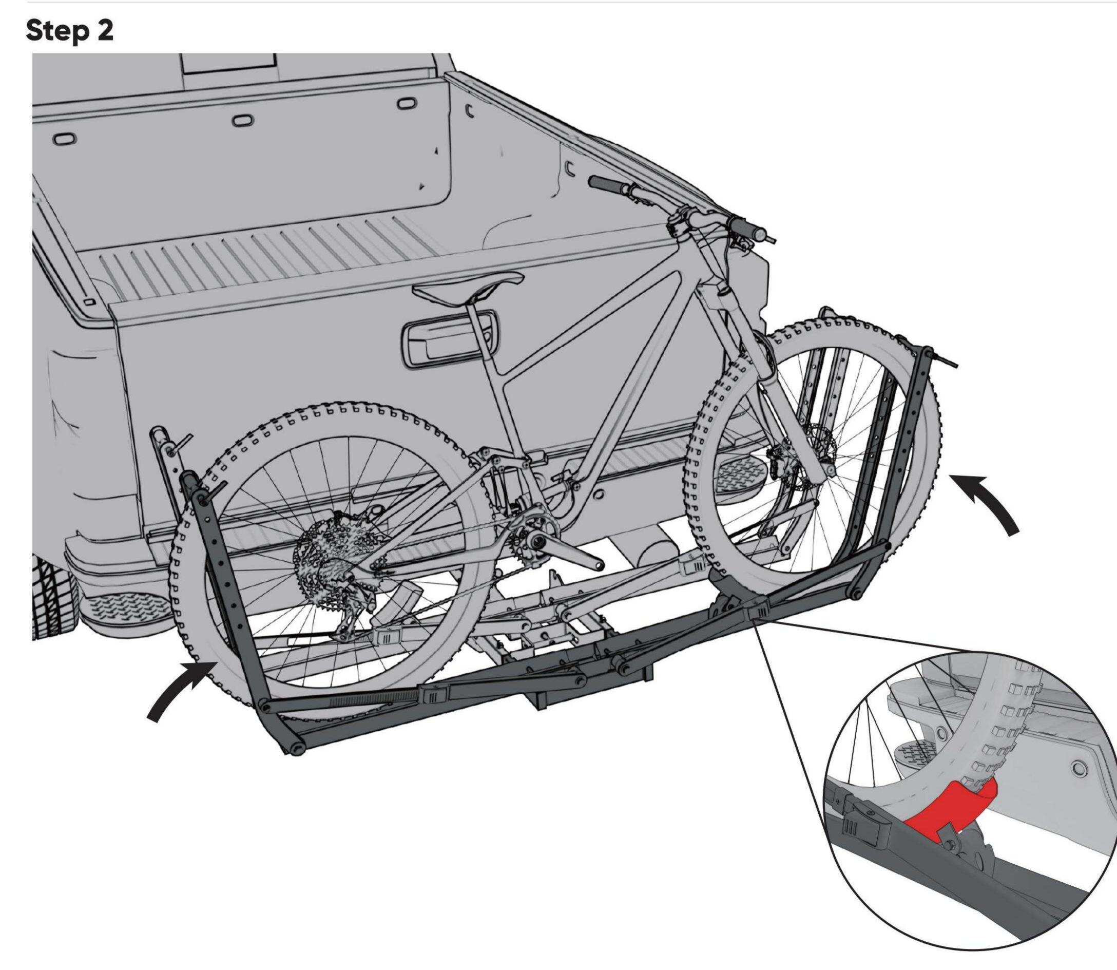
Install the bicycle on the Bike Rack, place the front wheel against the Front Wheel Holder, and tighten the Bent Arms on both sides to ensure that the front and rear wheels of the bicycle are firmly fixed.
