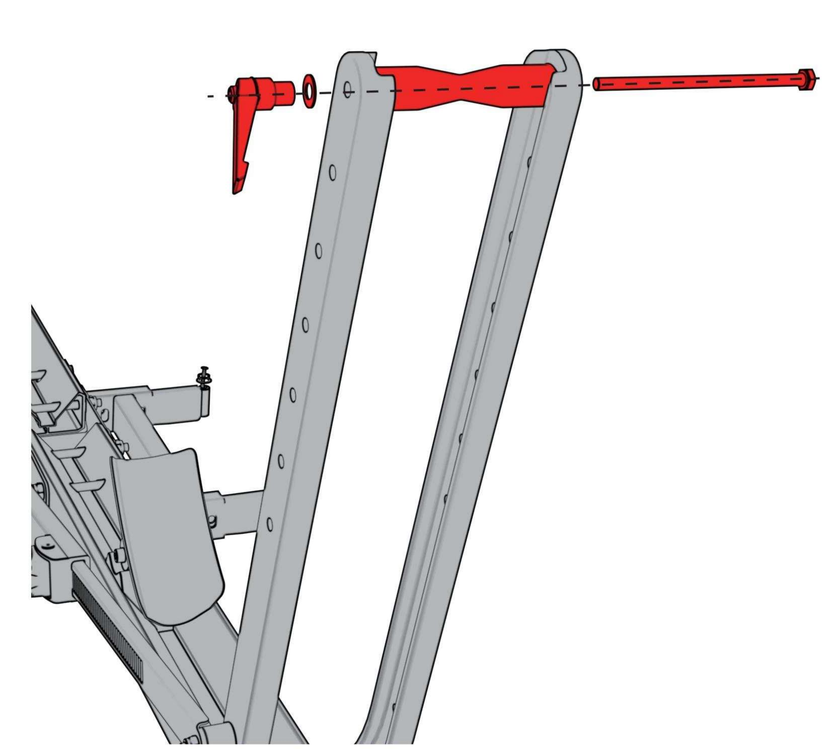
The position of the Adjustment Lever can be adjusted according to your needs. Loosen it counterclockwise and tighten it clockwise.
