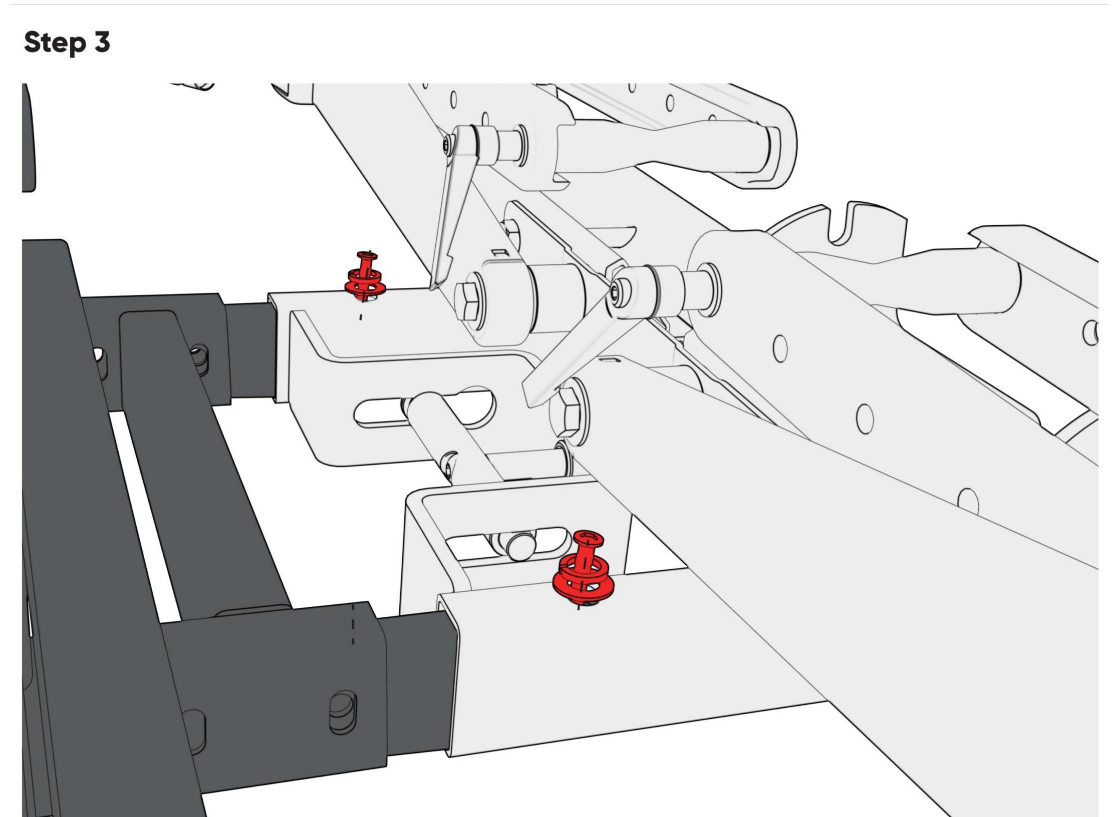
Bolt the connection assembly onto the MagRack X1 product.
