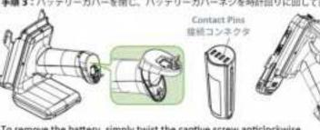
To remove the battery, simply twist the captive screw anticlockwise and take the battery out.
