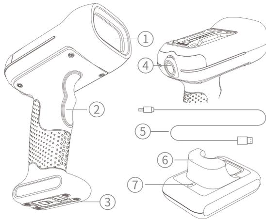
**EN:** ① Barcode Scanner ② Scan Button ③ Charging Port ④ Power Button ⑤ USB Cable ⑥ Base ⑦ Base Indicator
