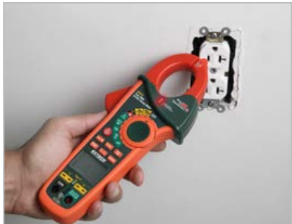
Non-Contact Voltage (NCV) Detection.
