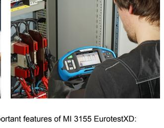
• Over 40 single tests (ranging from basic voltage, current measurements to illumination and phase sequence measurements)
