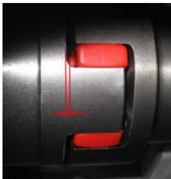
1. Coupling distance (check before disassembling)
