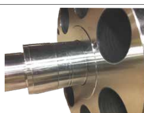
4. Place where shaft is screwed into barrel
