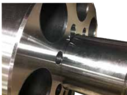
5. Place where shaft is screwed into barrel
