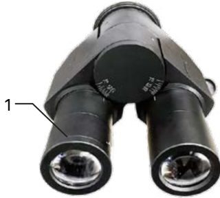
Fig. 10. Adjusting the diopter adjustment mechanism
