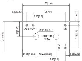
Case No.IRM03 Unit:mm[inch] Tolerance:±0.5[±0.02] unless otherwise specified
