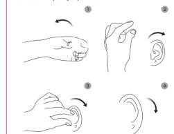
When the phone is connected, press and hold for 2 seconds to wake up the voice assistant (both left and right earphone can operate).
