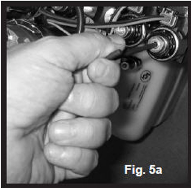
Fig. 5a Clockwise for manual override
