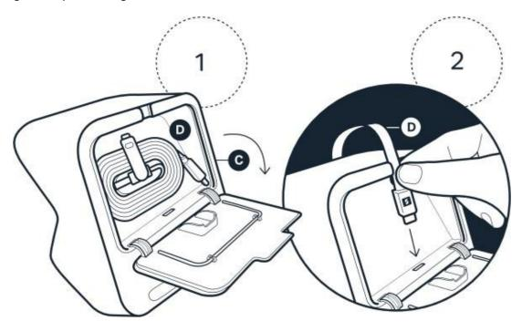
To charge SumUp Solo using the USB 2.0 type C cable directly
