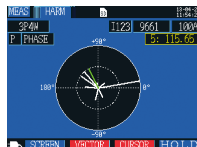
Harmonic power phase angle graph screen
