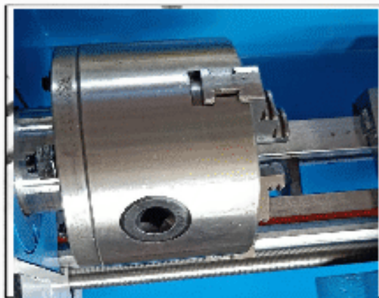
Fig. 7 Replacement Of Jaws
