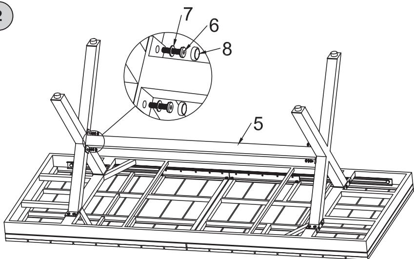
**Note:** Once all the screws are in place, they can be fully tightened.
