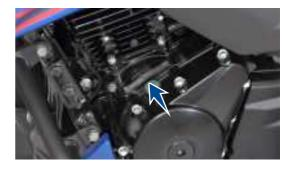
Engine serial number is engraved on the left side crankcase assembly near the cylinder block as shown.
