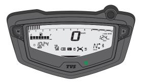
Once the cluster is connected with the smart phone, the cluster displays the signal strength of the network provider 'IIII' and the battery level 'IIIII' of the smart phone. Number of unread messages ' IIIII' and number of missed calls 'III' 5 '.
