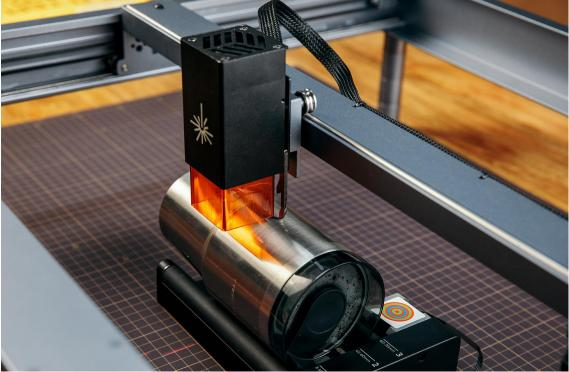
(2) Move the laser head again to position the center of the cross-shaped light beams at the start point to be engraved.
