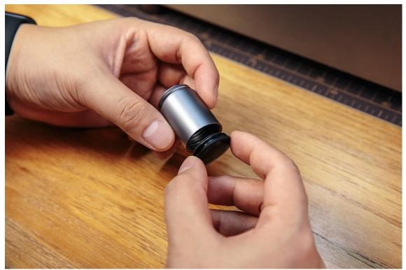
(3) Fit the cylindrical spacer blocks to the supports of Laserbox D1.
