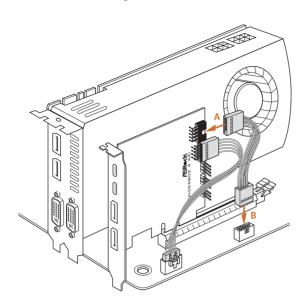
6. Connect one end of the DisplayPort Cable to the **DisplayPort IN Port (DP\_1)** (A) on the Thunderbolt 4 AIC R2.0. Then connect the other end of the cable to the **DisplayPort Port (B)** on the motherboard's rear I/O panel or on the graphics card.
