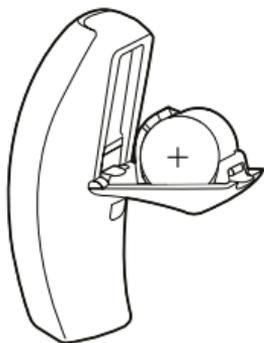
When the hearing aid is not in use, keep it in a warm, dry place with the battery drawer open to ventilate the hearing aid and allow it to dry.
