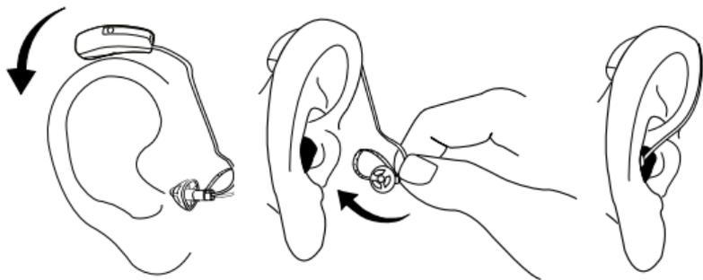
The illustrations show an open ear-tip. For further information on ear-tip types, anchors and procedures, see the separate ear-set user manual provided.
