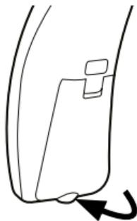
Use the nail grip to gently swing the battery drawer open. Do not press the drawer beyond the open position.
