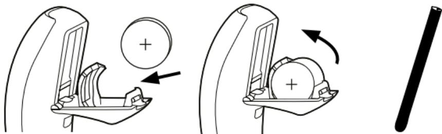
If the battery drawer does not close easily, the battery is incorrectly inserted.
