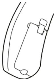
The battery drawer of the hearing aid also functions as the on/off switch.
