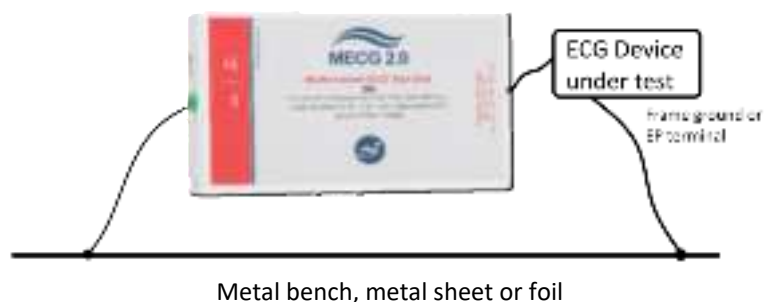
Figure 2: Set up a noise-free test environment
