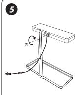
Fix the lighting Screw out the screw and washer of the lighting panel. panel with screw and washer.
