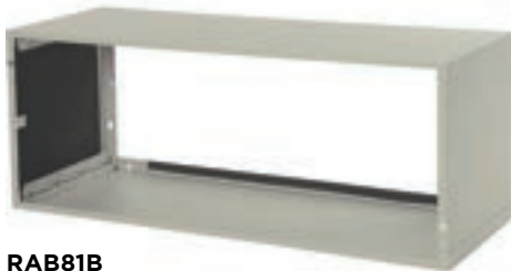
RAB81B WALL SLEEVE • Universal design • Insulated top & sides • Heavy gauge metal • Color matched • 4-piece "quick snap" design • Ships fully assembled
