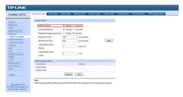
Step 3: Enable IGMP Snooping for port 1,2,3,4 in "Multicast-IGMP Snooping-Port Config". Please note port 5 is not needed for IPTV services, so we do not enable port 5 for IGMP snooping. If the desktop computer is also to receive the multicast service, Just Enable port 5.
