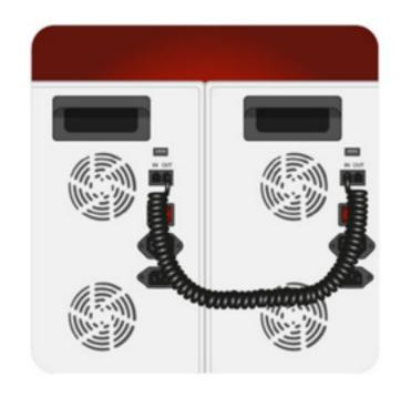
Repeat this process with the jumper power cables going from the main panel to the following panels.
