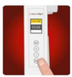
From the Home Screen press 'SET' to navigate to the Settings Screen. To adjust the Default Time, Mode, Bluetooth connectivity, and Brightness settings press 'SET'.
