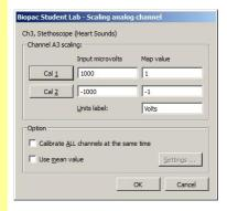
**Scaling** allows you to easily translate the voltage read by the MP hardware into the units being measured. Note that, for CH3, Stethoscope (Heart Sounds,) the Units label has been changed to "Volts."
