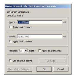
The **vertical scale** at the right edge of the graph window displays the amplitude units and range for each channel.
