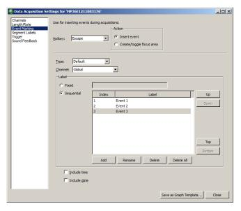
Event Marking setup offers options for assigning function keystrokes used to insert particular event types, and/or pre-defined event labels. This allows you to **pre-establish custom labels** *before* recording that are entered when an event is inserted *during* recording. This is helpful for entering various event types with descriptive labels during recording at exactly the moment an event occurs, when you otherwise might not have time to label them.
