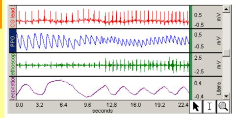
To optimize the horizontal scale for <u>all</u> waveforms and make all the data visible in the graph, choose the menu command **Display > Autoscale Horizontal**. This sets the horizontal (time) scale range to start at 0 (beginning of acquisition) and end at the end of the recording. The entire recording is displayed.
