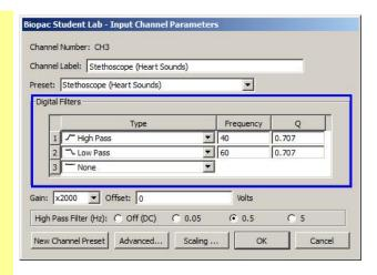
The MP unit hardware-based **Digital Filters** are three cascading, second-order filters that can be set independently using the pull-down boxes. They are designed primarily for basic signal conditioning (e.g., removing 50/60 Hz noise,) rather than for filtering data to retain physiological signals of interest (such as retaining alpha activity from an EEG signal). Specify a **filter type** (low pass, high pass, band pass, or band stop.) **frequency,** and **Q setting**.
