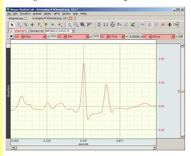
You may also average a selected portion of the recording. This feature is useful when comparing the ECG complex during different sections of an experiment.
