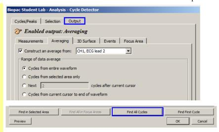
BSL PRO runs through the data and generates a new graph window showing the **average ECG** for the entire recording.
