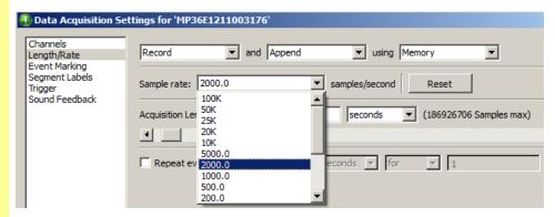
The three pull-down menus at the top of the **Acquisition setup** dialog allow control over the recording mode and where the acquisition data will be saved.
