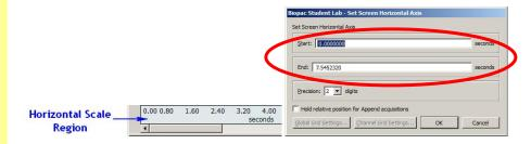
The **horizontal scale** can be adjusted to any range to compress or expand the displayed waveforms along the horizontal (time) axis. **The horizontal scale affects all channels.**
