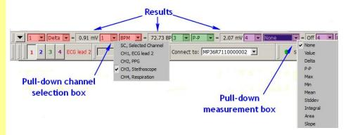
The **measurement region** is located near the top of the graph window. For each measurement, there are pull-down boxes that specify the channel to be measured and type of measurement, and a value box that displays the results.
