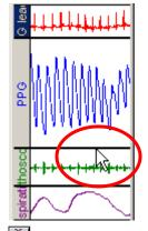
You may use the Arrow tool to adjust chart boundaries and better view a waveform's "track." Position the Arrow tool over a boundary line between waveforms. When the cursor changes style, drag to resize the track of that waveform. (The I-Beam tool similarly changes style and can be used to adjust chart boundaries.)
