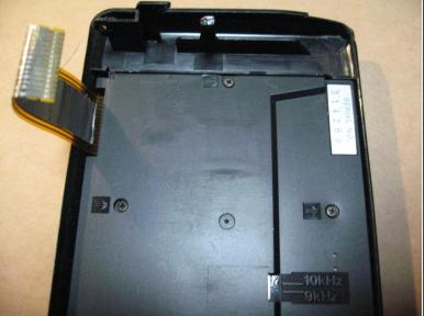
Now gently pry the door hinges on either side off of their pivot point, and remove the front door from the assembly
