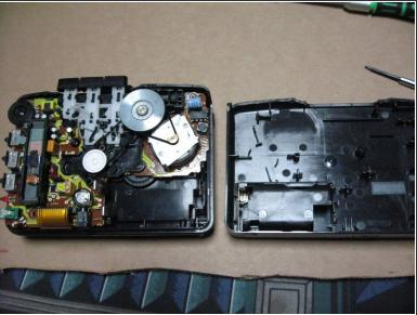
Take care not to jostle the Switches on the top of the unit while removing case. So now we have removed the underside casing from the device.
