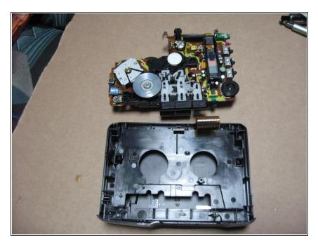
Now we can remove the board from the casing.
