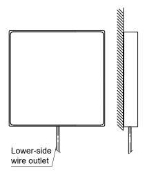
Inside wall wiring (with an 86-type box)
