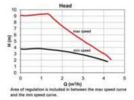
Available external static pressure VS Flow rate
