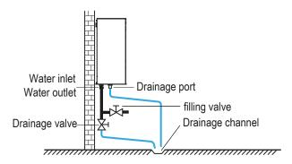
When water is at standstill inside the system, freezing is very likely to happen and damage the system in the process.
