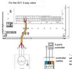
\* - In the case of using an actuator with a constant control voltage on one wire, it should be connected to terminal number 15 (L1) on CN11.
