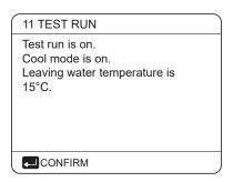
During COOL MODE test running, the default target outlet water temperature is 7°C. The unit will operate until the water temperature drops to a certain value or the next command is received.
