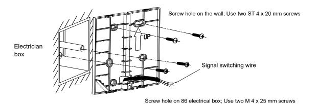
• Buckle the front cover, and fit the front cover to the back cover properly, leaving the wire unclamped during the installation.
