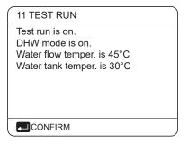
During DHW MODE test running, the default target temperature of the domestic water is 55°C. The TBH(tank boost heater) will turn on after the compressor runs for 10min. The TBH will turn off 3 minutes later, the heat pump will operate until the water temperature increase to a certain value or the next command is received.
