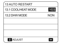
The AUTO RESTART function reapplies the user interface settings at the time of the power supply failure. If this function is disabled, when power returns after a power supply failure, the unit won't auto restart.
