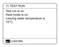
During HEAT MODE test running, the default target outlet water temperature is 35°C. The IBH (internal backup heater) will turn on after the compressor runs for 10 min. After the IBH runs for 3 minutes, the IBH will turn off, the heat pump will operate until the water temperature increase to a certain value or the next command is received
