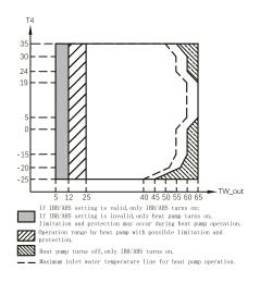
In DHW mode, the water flowing temperature(TW\_out) range in different outdoor temperature(T4) is listed below:
