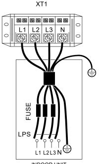
INDOOR UNIT POWER SUPPLY Three-phase 3/6/9 kW heater
