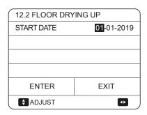
During floor drying, all the buttons except  $\Lappa$  are invalid. When the heat pump malfunctions, the floor drying mode will turn off when the backup heater and additional heating source is unavailable. If you want to turn off floor drying up, please press  $\Lappa$ . The following page will be displayed:
