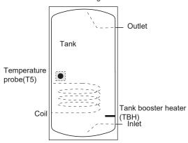
The booster heater should be installed below the temperature probe (T5).
